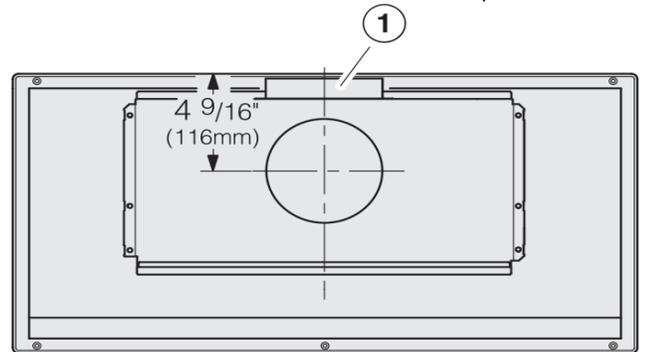
① The ducting can also be connected at the back.
