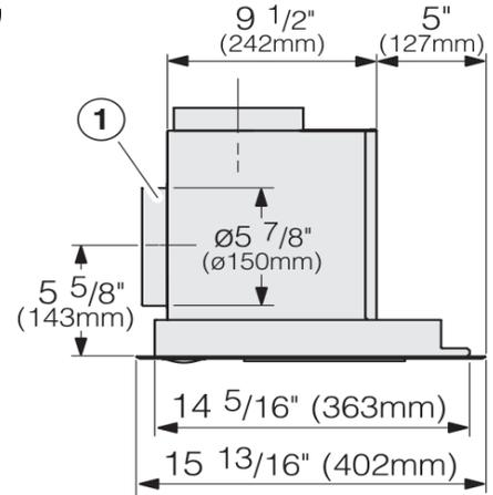
① The ducting can also be connected at the back.
